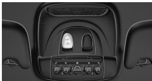
SOS button in the roofliner
